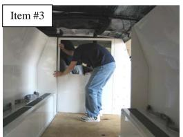
Attach Front Bulkhead to Driver-side Bench/Wall assembly
